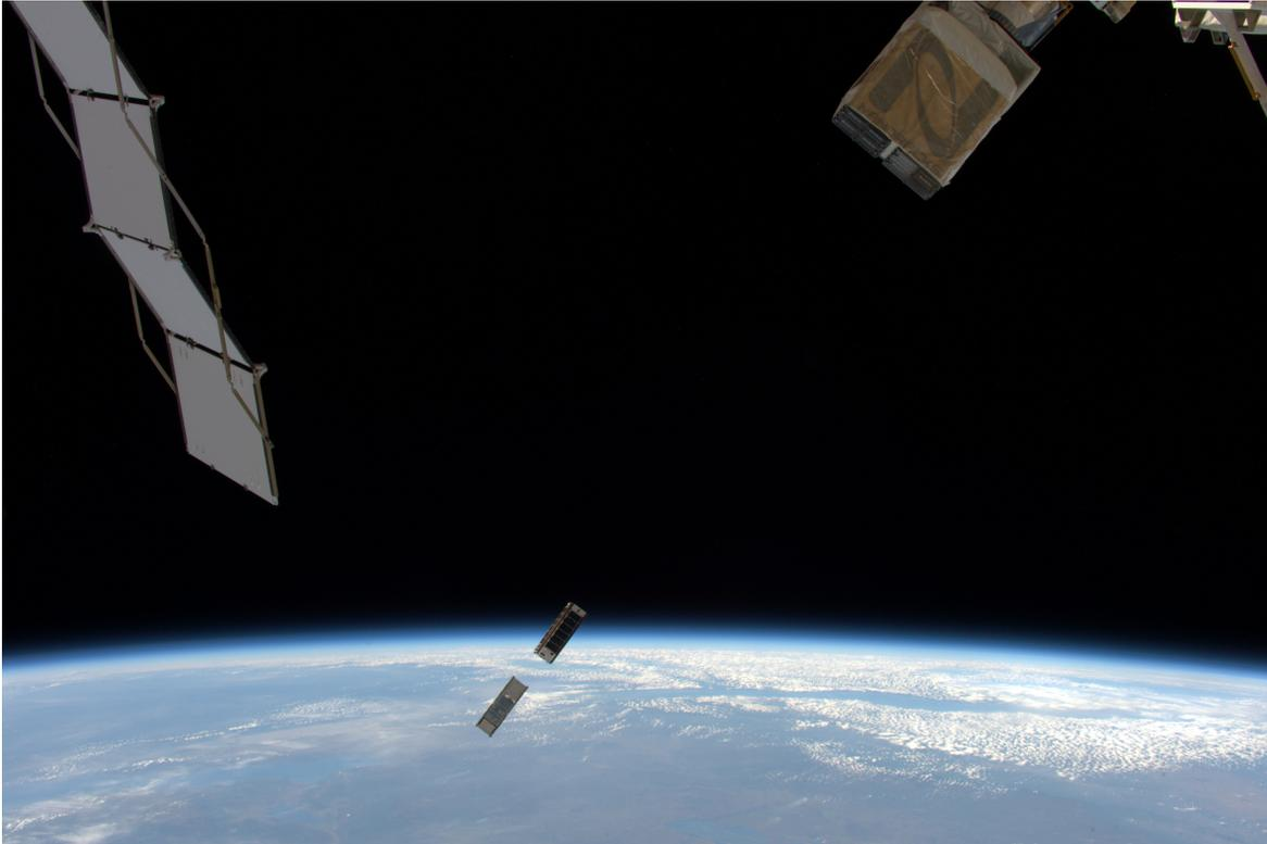
*Astronaut Tim Peake on board the International Space Station captured this image of a CubeSat deployment on May 16, 2016. The bottom-most CubeSat is the NASA-funded MinXSS CubeSat, which observes soft X-rays from the sun—such X-rays can disturb the ionosphere and thereby hamper radio and GPS signals. (The second CubeSat is CADRE — short for CubeSat investigating Atmospheric Density Response to Extreme driving - built by the University of Michigan and funded by the National Science Foundation.)*
