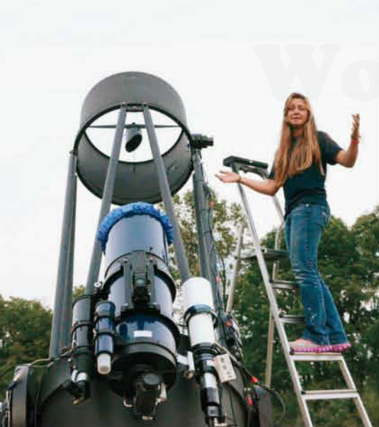
Co-author Emily A. Mailhot poses atop an observing ladder to lend a sense of scale to the 25-inch Newtonian reflector.
