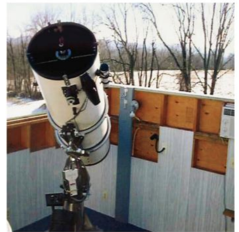
The first telescope housed in the rooftop observatory was this 16-inch f/5 equatorially mounted Newtonian reflector. After a few years of using it, Midkiff sold it and purchased a 25-inch reflector.
